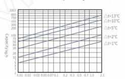
Pressure Differential MPa  $\Delta t$ = Setting temperature-Valve actual drainage temperature
